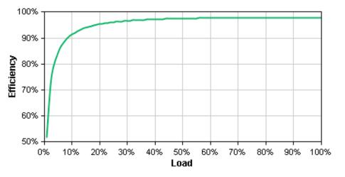
Curve fit to measured efficiency data. All measurements taken in normal operating mode, at typical environmental conditions, with nominal electrical input and balanced resistive load (PF = 1.0) output.
